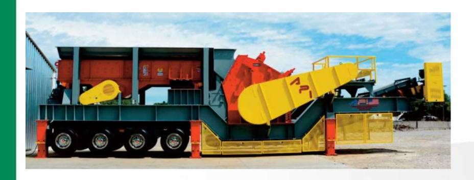
Image: Electric rock crushing using electricity in Illinois (Coles-Moultrie) increases co-op load, improves operation, and reduces air pollution
