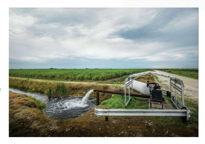
In 2014, PERC partnered with engine manufacturers, California equipment dealers, and growers to test the performance of propane-powered engines in the state. Eight units were placed in fields to irrigate a variety of crop types, including rice, wine grapes, feed for dairy cattle, fruits, nuts, and vegetables for one growing season.
